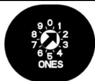
Figure 31: B426 Switch Set to Address 1
