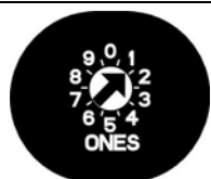
Figure 32: B420 Switch Set to Address 1
