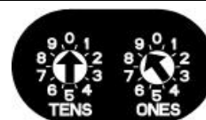
Figure 30: B308 Switches Set to Address 9
