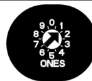
Figure 35: B820 Switch Set to Address 1
